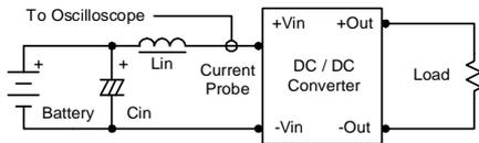
**Peak-to-Peak Output Noise Measurement Test**
