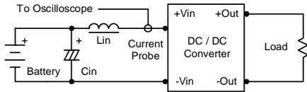
**Peak-to-Peak Output Noise Measurement Test**
